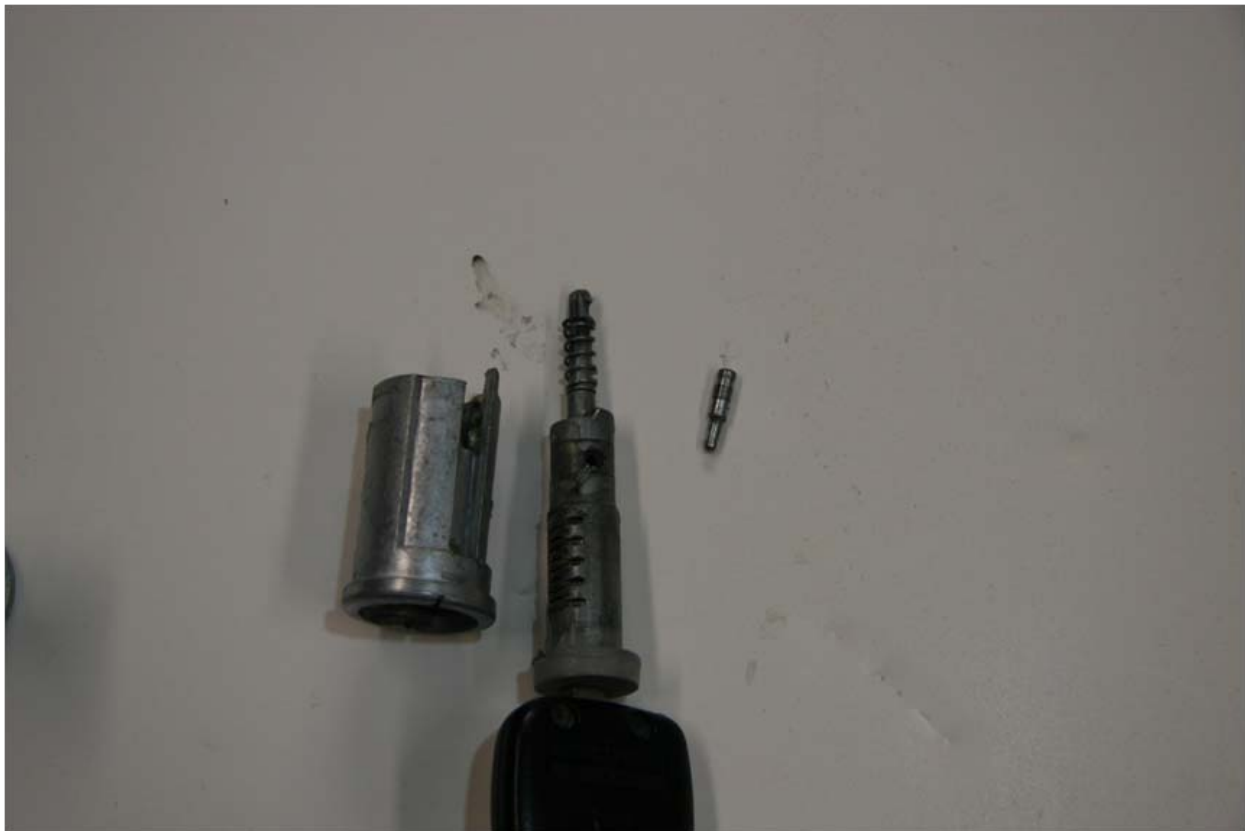
Lock Removed from Cylinder
